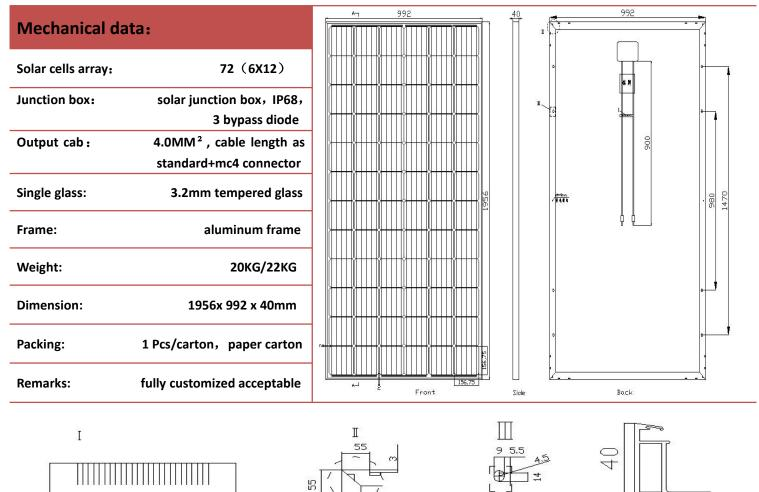
Specially designed for the medium and large scale use of power, with high stability and long term life time of correct use, which could provide power for a family, or even a committee, for the daily use of power. Together with battery and inverter we could install a small pv plant for a home, and with large quantity of our solar modules, we could also install giant pv plant even for an area. It is your smart choice to be with us!
